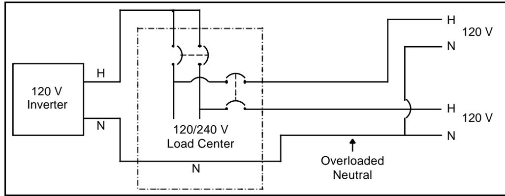
**Figure 23. Diagram of a Multiwire Branch Circuit**
