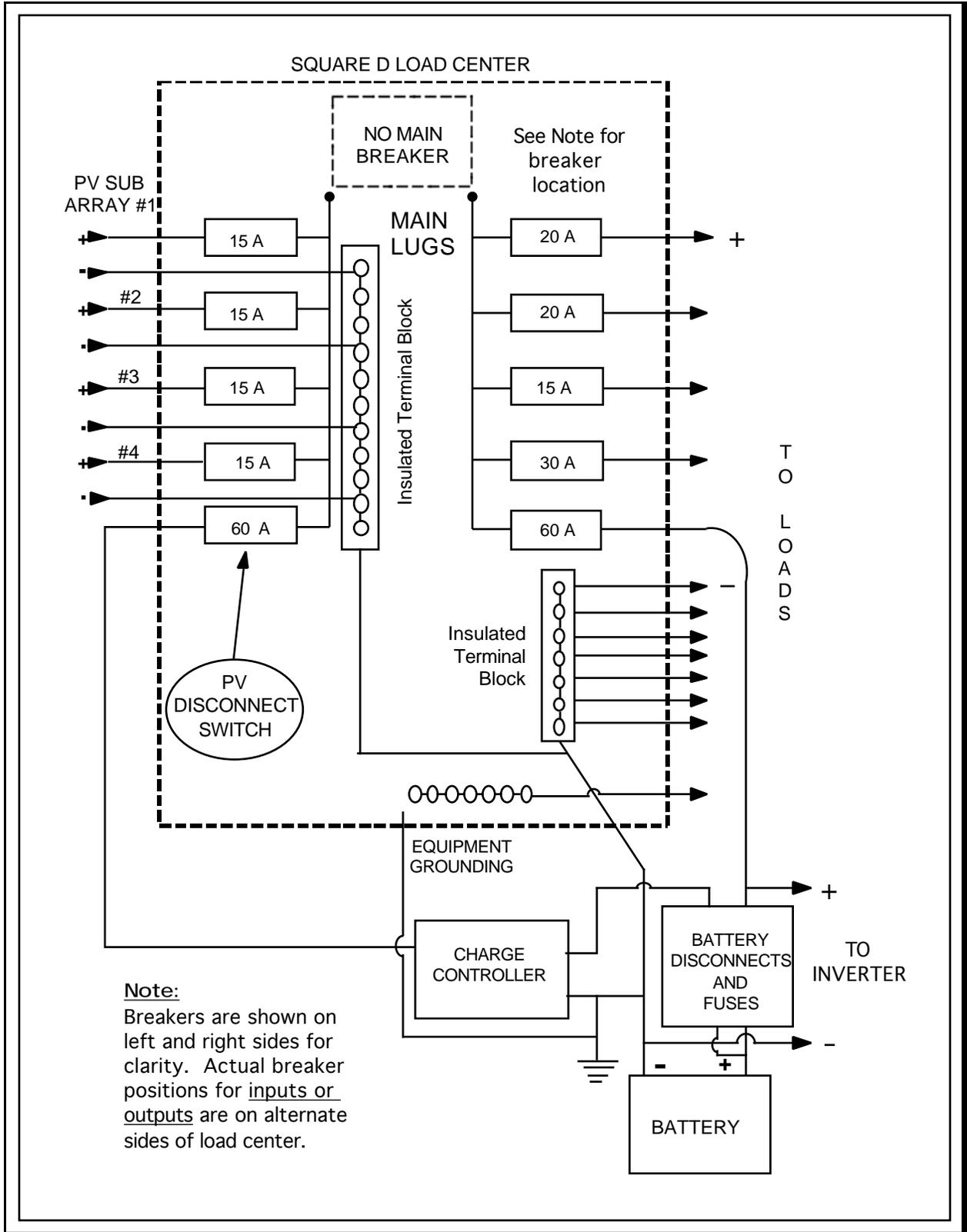
Figure 21. 12-Volt DC Combining Box and Load Center
