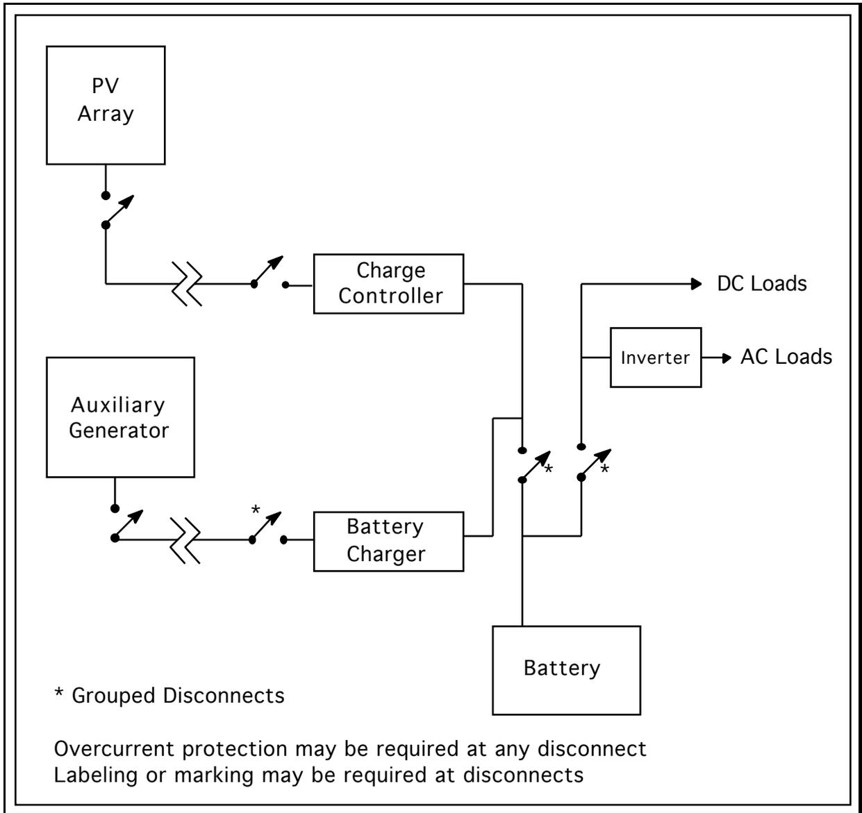
**Figure 18. Disconnects for Remotely Located Power Sources**
