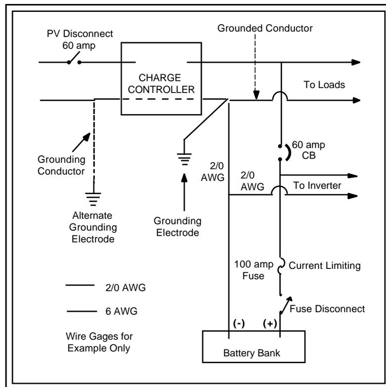
**Figure 8. Typical System: Possible Grounding Conductor Locations**
