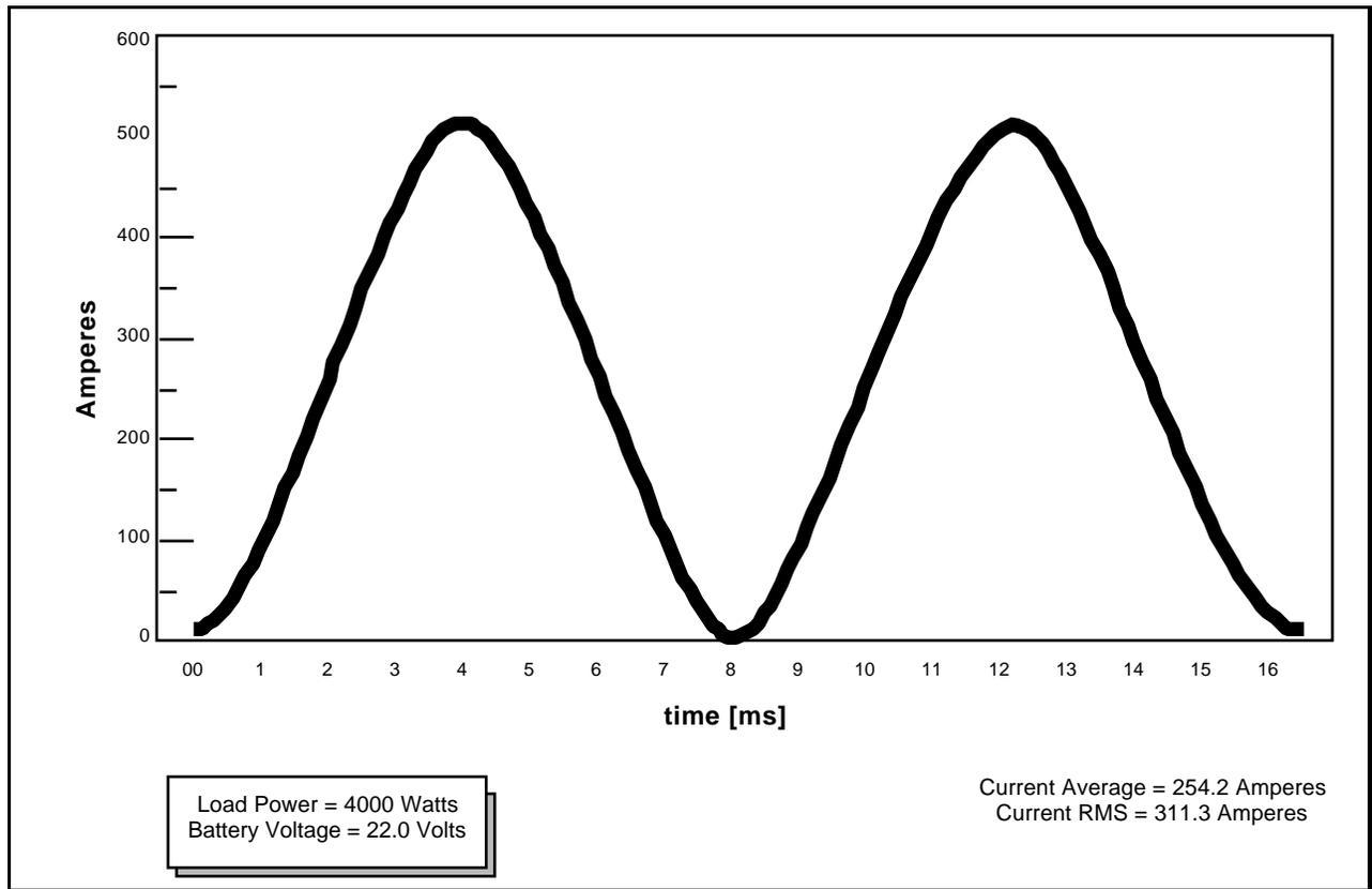
**Figure F-1. Inverter Current Waveform (dc side)**
