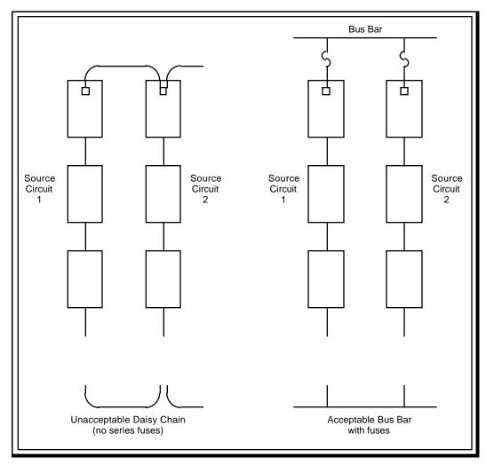
Figure 6. Module Interconnect Methods
