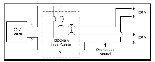
Figure 23. Diagram of a Multiwire Branch Circuit
