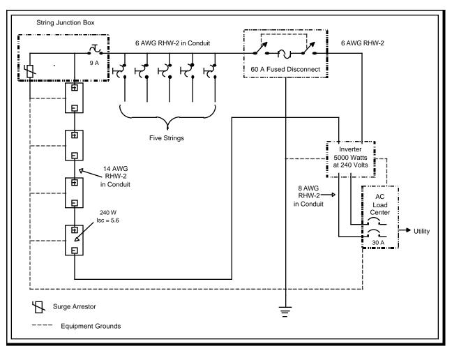
Figure E-7. Roof-Top Grid-Connected System
