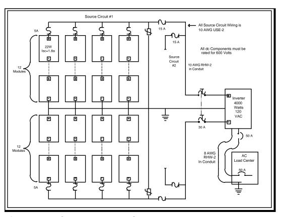
Figure E-8. Center-Tapped PV System
