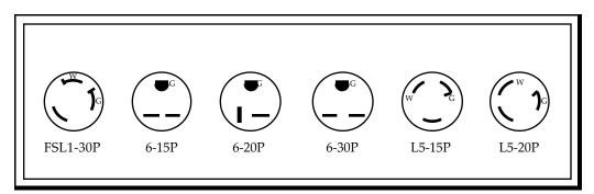
Figure 22. NEMA Plug Configurations
