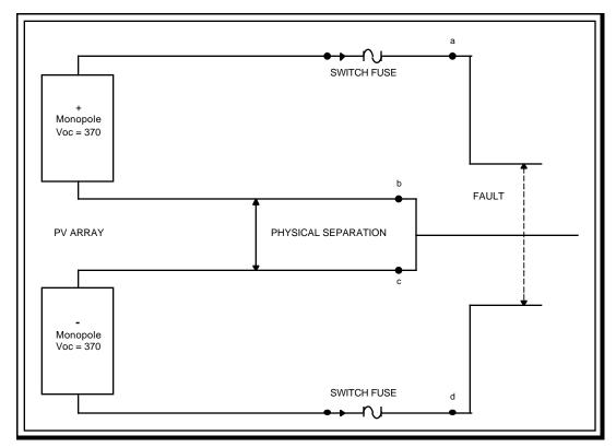
Figure D-1. Typical Bipolar System with Fault
