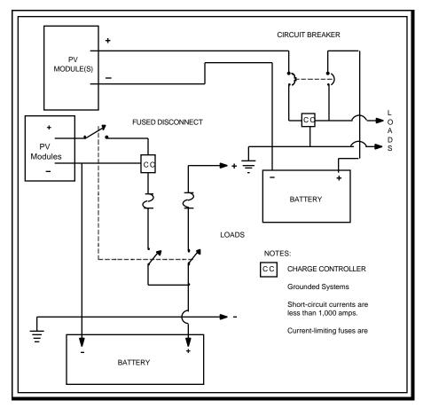
Figure 15. Small System Disconnects
