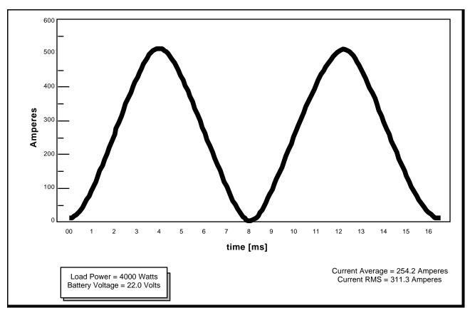
Figure F-1. Inverter Current Waveform (dc side)
