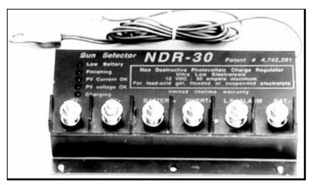
Figure 19. Typical Charge Controller
