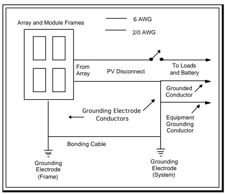
Figure 9. Example Grounding Electrode System
