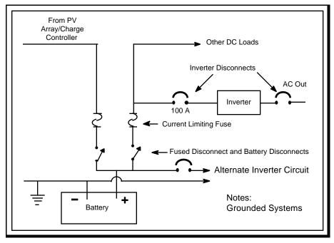
Figure 16. Separate Battery Disconnects
