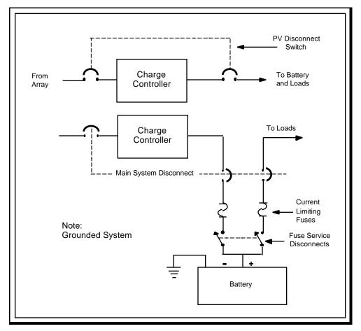
Figure 17. Charge Controller Disconnects
