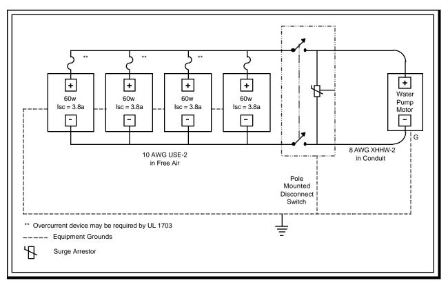
Figure E-1. Direct Connected System
